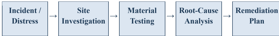
Figure 4.13 A typical structural failure investigation process.
